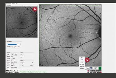
Select **BAF** from the software menu or via the touch panel (**FA/BAF**) and double-check the image is focused properly.
