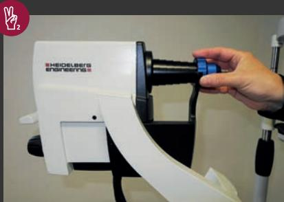
Turn the focus knob to approximately +21 diopters and pull the camera backwards. Insert the ASM by aligning the red dots of the camera head and the ASM. Turn the ASM about 50° clockwise until it catches.
