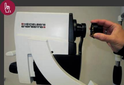
Turn the 30° SPECTRALIS standard lens about 50° counterclockwise and remove it.
